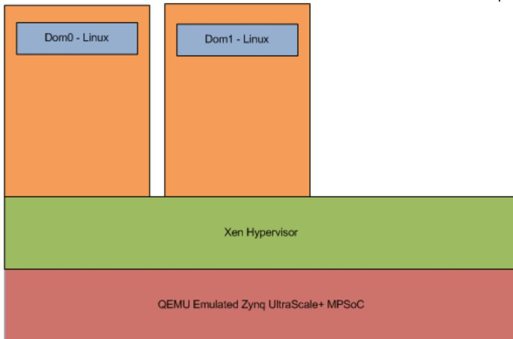
**Figure 2. System Architecture**
